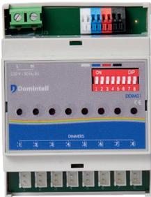
The DDIM01 is the control module of 1 to up to 8 dimmers of 400 W (DD400L), 500 W (DD500), 750 W (DD750), 1000 W (DD1000) or 0-10 V/1-10 V (DD10V). This module simultaneously manages the dimmers with different power and tensions.
